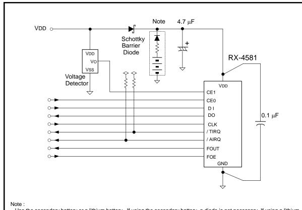
Use the secondary battery or a lithium battery. If using the secondary battery, a diode is not necessary. If using a lithium battery, a diode is necessary. For information on resistance value, please consult the battery manufacturer.
